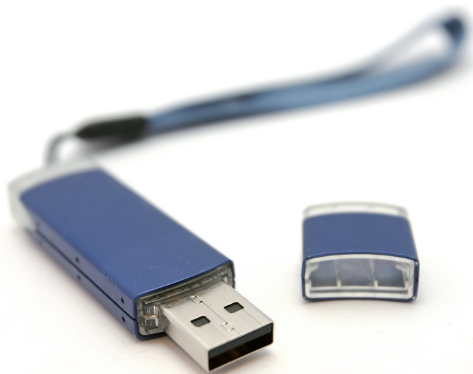
USB sticks typically hold several gigabytes of data. This one holds up to 16GB of storage.
